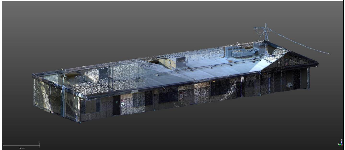
Here is an image of the point cloud data stripped of everything except the DDGT building.
