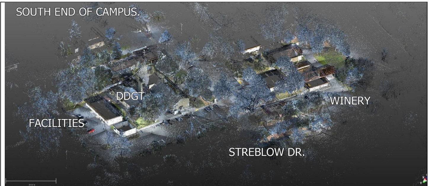
Here is an image of point cloud data of the South end of campus.
